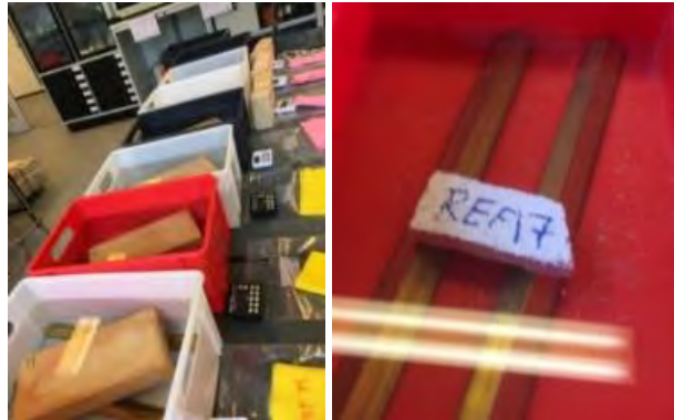
Figure 5-1: Experimental setup of full immersion water absorption experiments on brick (left) and mortar (right).
