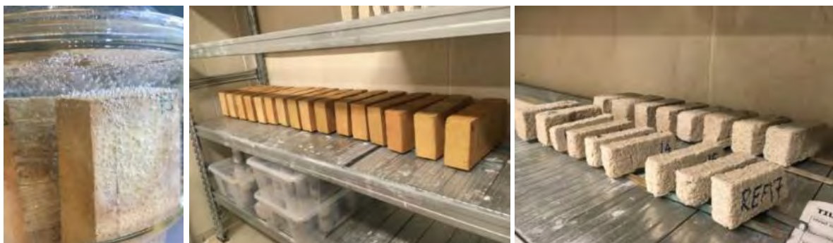
Figure 5-2: Vacuum saturation of brick in desiccator (left), and drying in climate chamber of brick (middle) and mortar (right).
