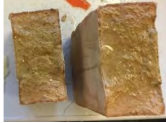
Figure 5-13: Impregnation depth of agent O on brick and mortar.
