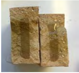
Figure 5-11: Impregnation depth of agent I on brick and mortar.
