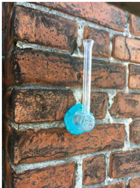
Figure 8-5: Karsten tube fixed on mortar joint
