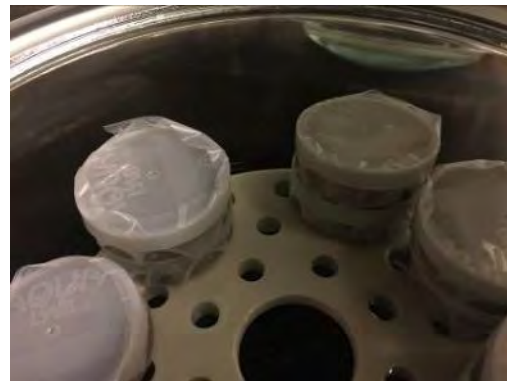
d. Samples sealed in cups
