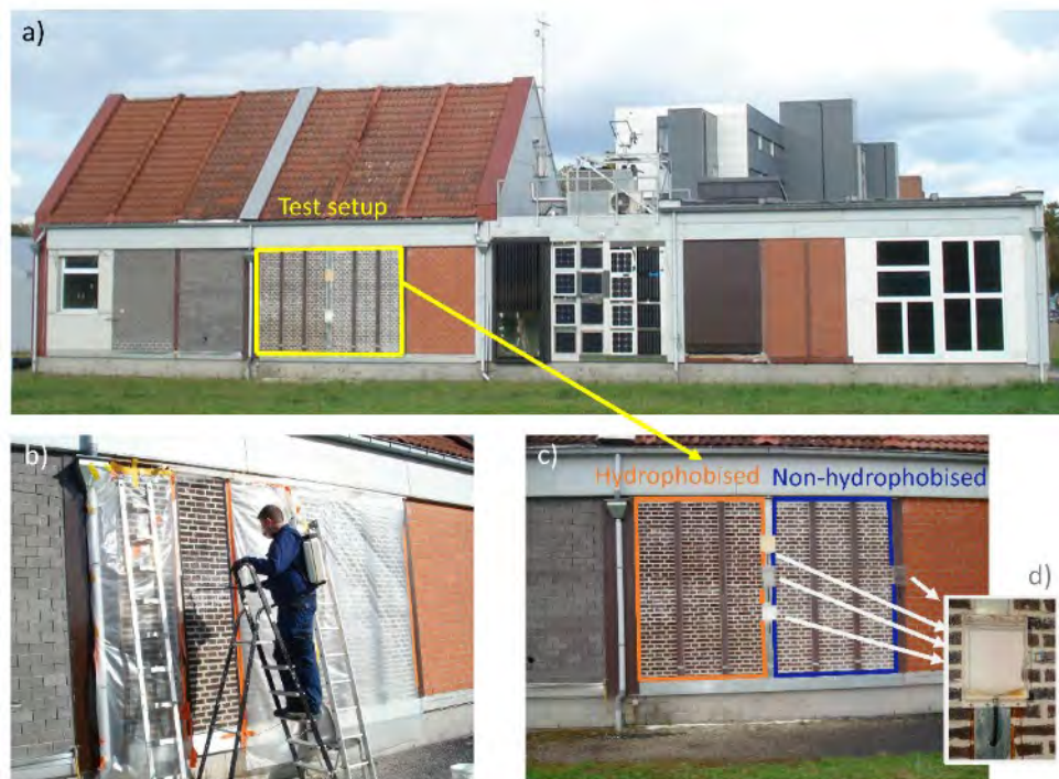
Figure 10-1: Outside view of the field test setup: (a) south-west oriented side of the VLIET-test building, (b) spraying of the hydrophobic agent solution, (c) hydrophobised and non-hydrophobised masonry test walls with (d) wind-driven rain gauges.
