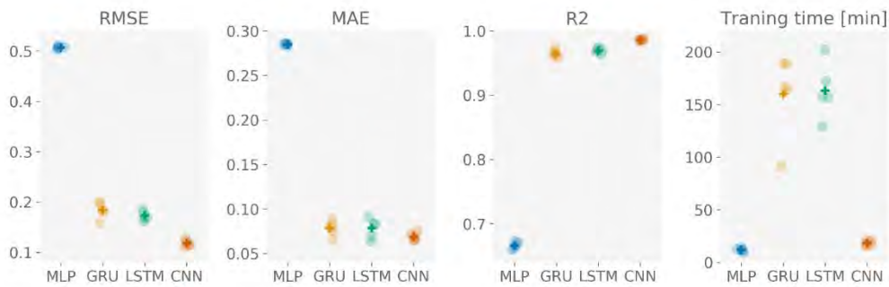
Figure 48: The performance indicators, calculated over all outputs together, and training time for each neural network type. The dots show the results of the five replications, while the crosses represent the average result.
