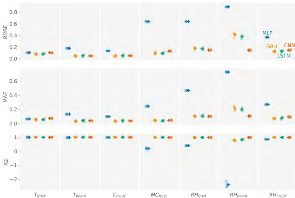
Figure 49: The performance indicators, calculated over each output separately for each neural network type. The dots show the results of the five replications, while the crosses represent the average result.
