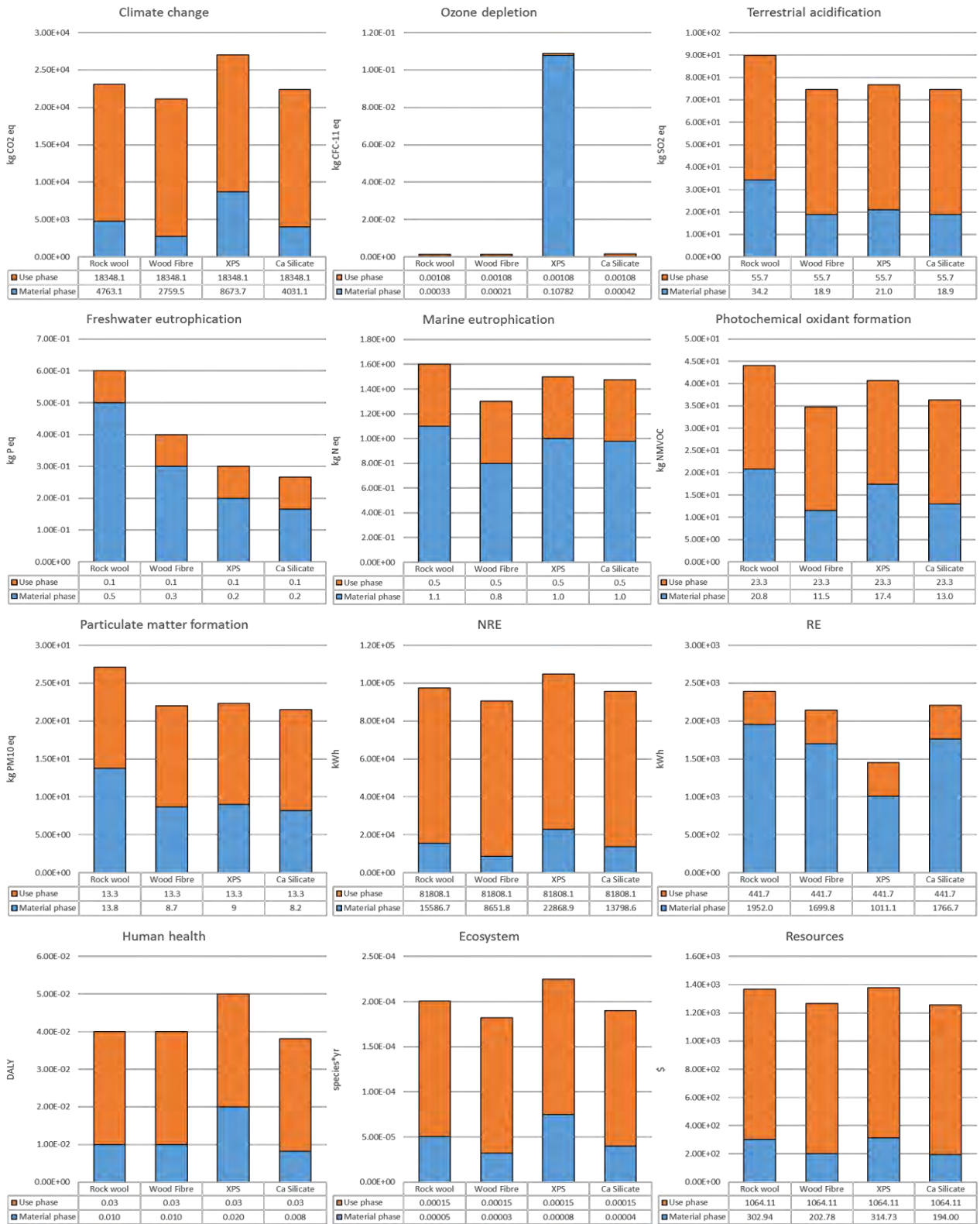
Figure 86 Life cycle analysis and comparison of the four design options for the selected environmental indicators considering the components level (use phase component)
