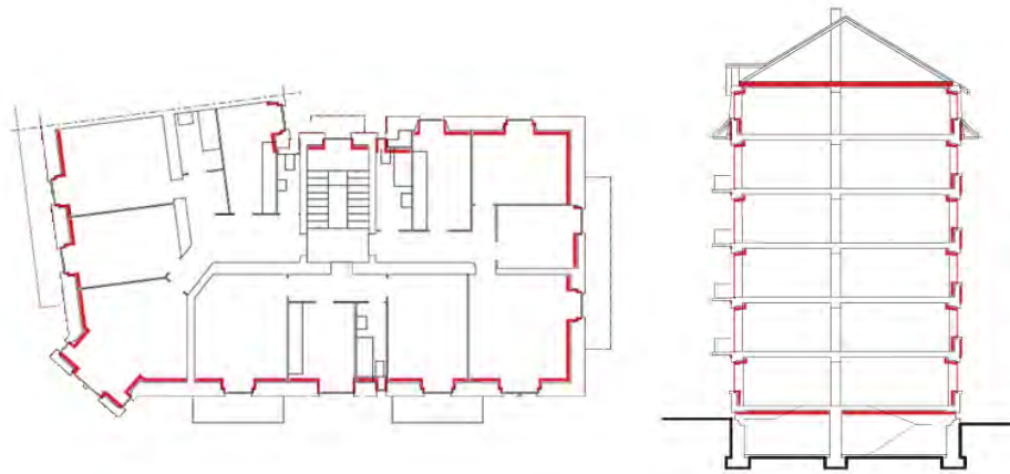
Figure 74 Renovation scenario 1, insulation added shown in red
