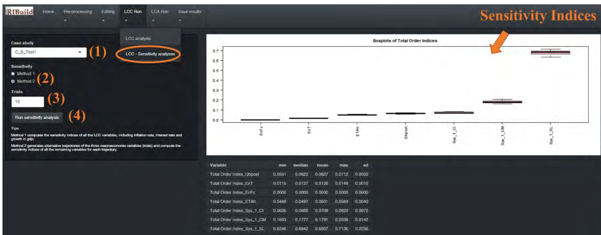
Figure 100 LCC Run menu → LCC – Sensitivity analysis. Calculation of the Sobol’s first order and total order indices for LCC inputs with Method 2
