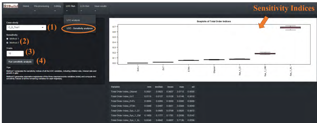
Figure 11 LCC Run menu → LCC – Sensitivity analysis. Calculation of the Sobol’s first order and total order indices for LCC inputs with Method 2
